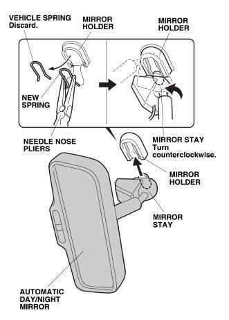
Slide the automatic day/night mirror stay into the mirror holder. Then turn the mirror stay counterclockwise to secure the automatic day/night mirror in the holder.  Using isopropyl alcohol on a shop towel, thoroughly clean the fuse case where the fuse label will attach. Attach the 2A fuse label to the fuse case on the automatic day/night mirror harness.
